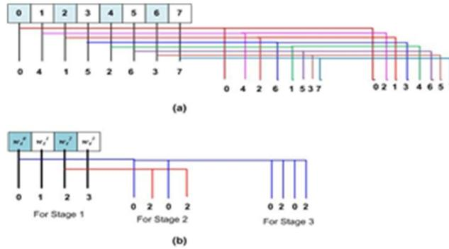
Fig. 4 Memory Representation. (a) Input Memory. (b) Twiddle Memory
