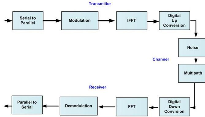
Fig. 2 Block Diagram of OFDM Software Defined Radio
