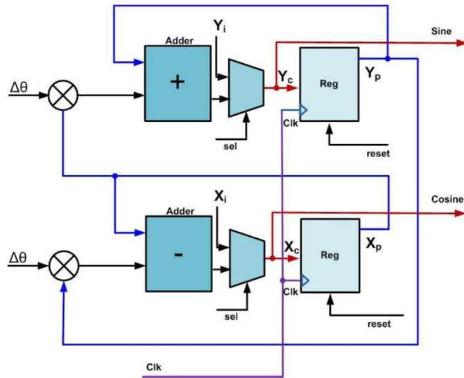
Fig. 7 The Proposed Architecture for DDFS
