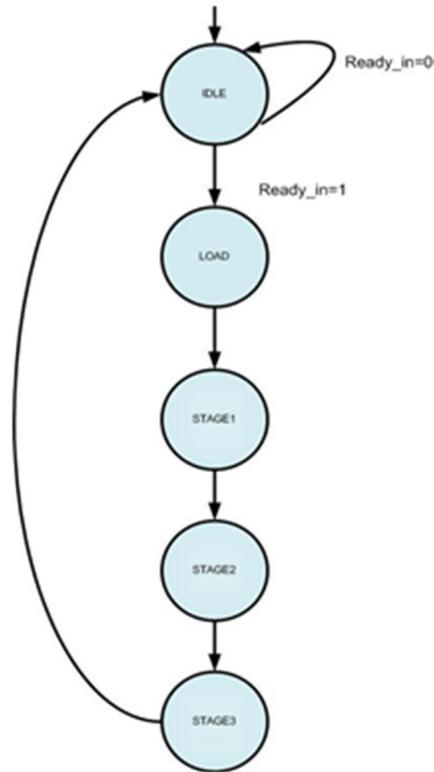
Fig. 6 State Transition Graph for FFT FSM
